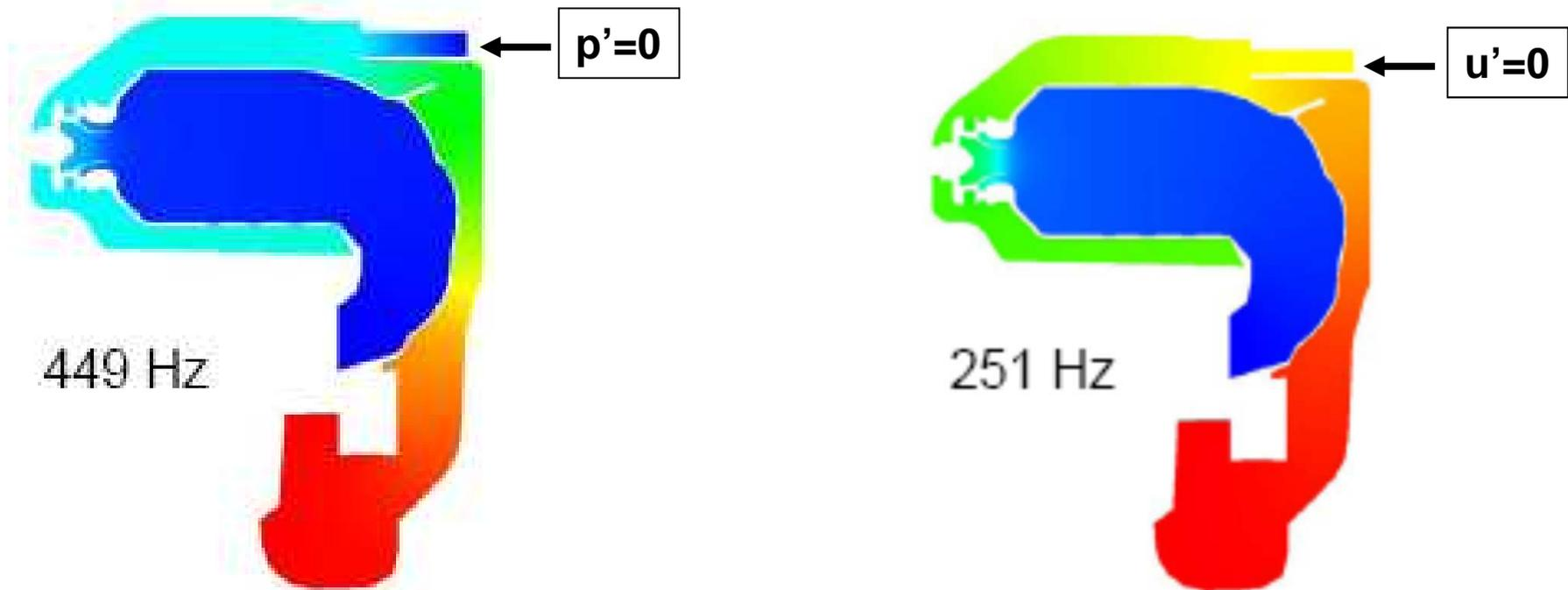
Acoustic analysis of a Turbomeca combustor including
